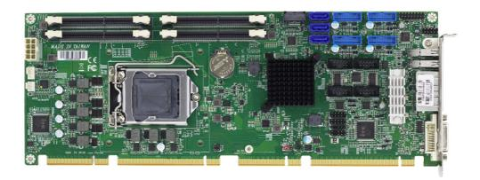
ROBO-8114VG2AR is based on Intel® C246 chipset and workstation processors. Built with flexible PCI express expansions, ROBO-8114VG2AR is suitable for Medical, Industrial Automation, and Digital Signage applications.
